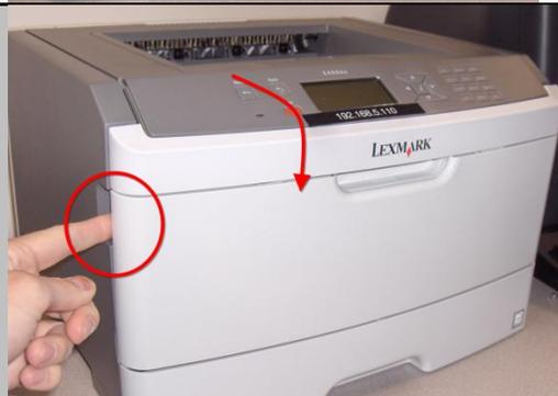
3. Grasp the handle and pull up and out to remove toner cartridge and photoconductor kit.
