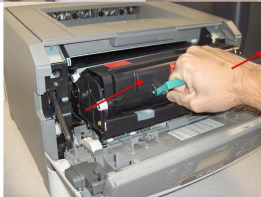
4. Separate the toner cartridge and photoconductor kit by pressing the release button on the PC Kit (circled) and pulling up and out.
