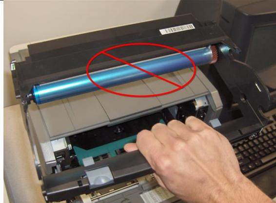
6. Install the toner cartridge back into the photoconductor kit. You should hear a click when the cartridge is completely pushed in.
