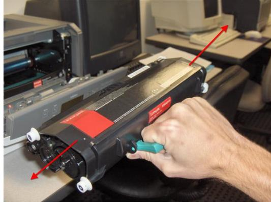
6. Install the new toner by aligning the white rollers on the cartridge with the white arrows on the tracks of the photoconductor kit. Push in the toner cartridge as far as it will go (you should hear a click).
