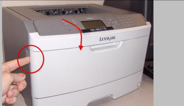
3. Press the release button at base of cartridge with thumb. Grasp the handle and pull up and out to remove the toner cartridge.
