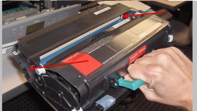
7. Insert the toner and photoconductor kit back into the printer.
